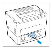
5 Remove the plastic strip from the rear of the printer.
